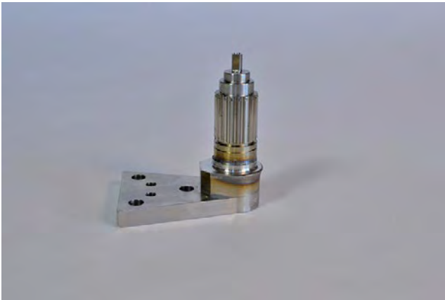
Figure 10. Friction welded gear part (1.4404).
