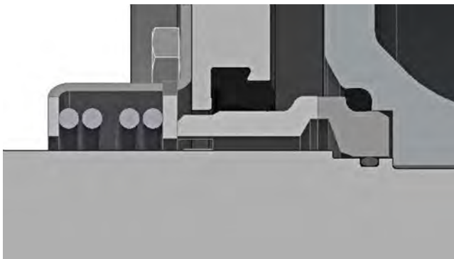
Figure 2. The design of the axial face seal in detail.
