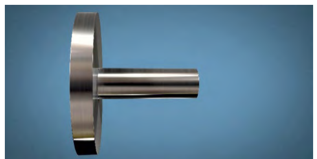
Figure 4. The flash is removed and the part is now ready for machining.
