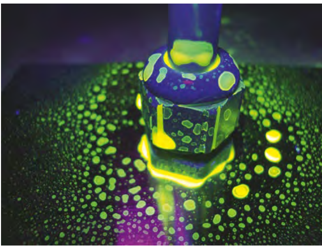
Figure 16. Standard plastic cable gland: after pressure rinsing – weak.
