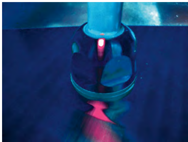
Figure 20. Pflitsch blueglobe CLEAN plus: after pressure rinsing – excellent.
