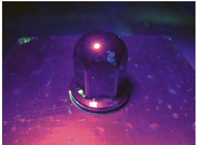
Figure 15. Novonox cap nut with flange incl. Hygienic Usit washer: after wiping – good.
