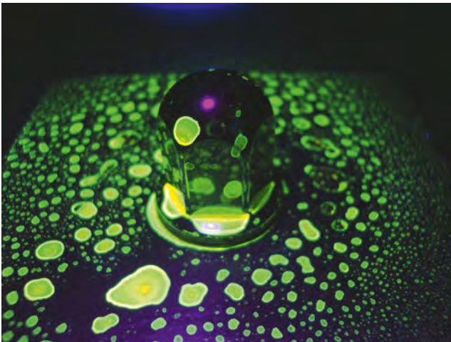
Figure 22. Cap nut with flange from Novonox with Hygienic Usit washer: after pressure rinsing – excellent.
