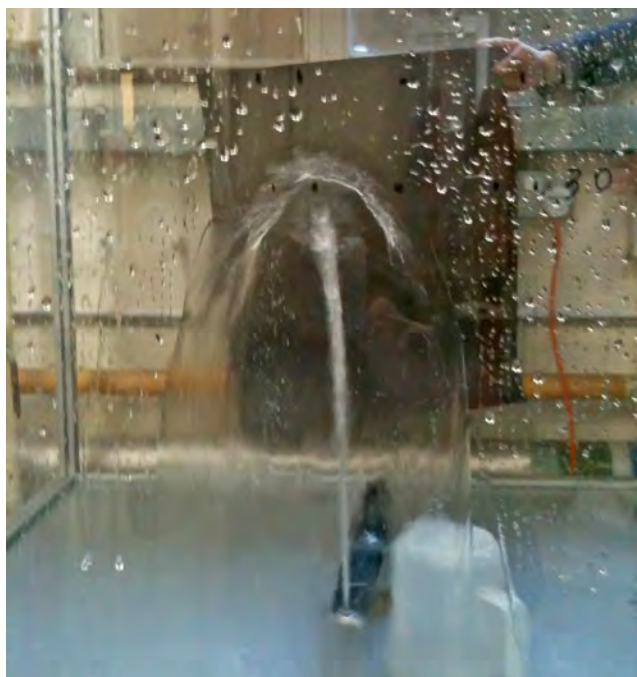
Figure 1. Upwardly inclined water jet impinging on a Perspex sheet. Radial flow zone, rope and draining film is evident. Operator hand in background provides scale.
