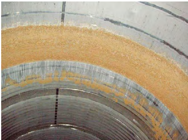
Figure 1. A hard-to-clean tub ring in a beer fermenter. (Photo courtesy of Sopura)
