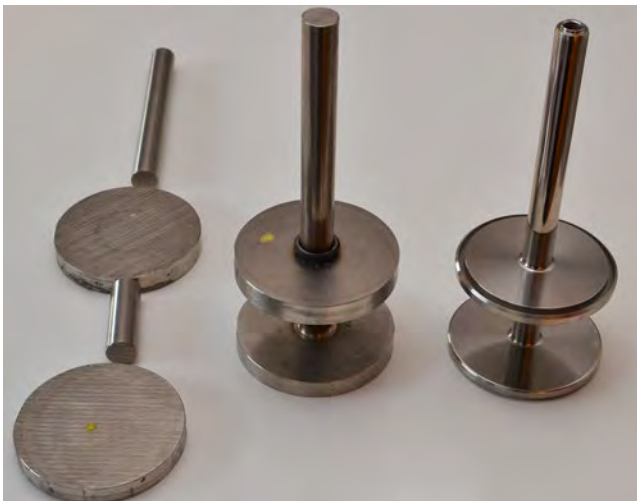
Figure 6. This double-seated valve (1.4404) is an example of a friction welded raw material to a finished machined valve.
