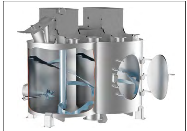
Figure 1. Twin shaft mixers create three-dimensional product flow, which eliminates dead spaces to improve hygiene.
