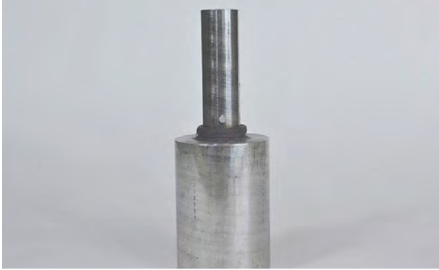
Figure 5. Pump shaft (1.4404 and 1.4301) can be friction welded.
