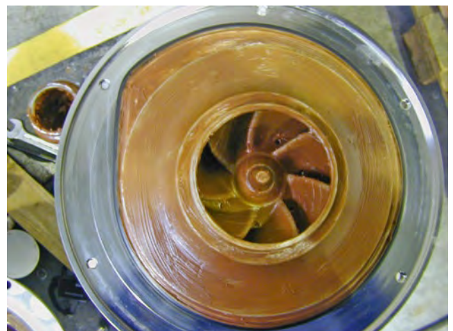
Figure 3. Preparation of a cleaning test on a closed impeller using chocolate paste.
