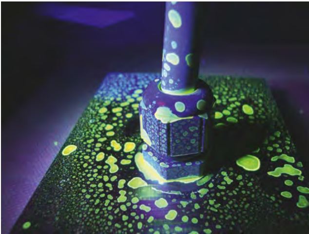
Figure 10. Standard plastic cable gland: after wiping – weak.
