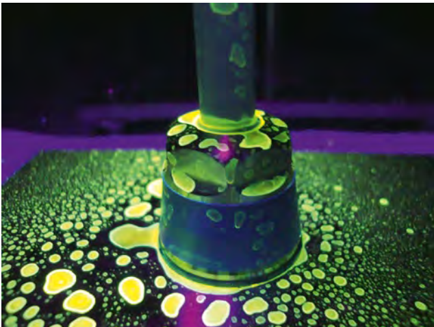
Figure 12. Pflitsch blueglobe CLEAN: after wiping – weak.
