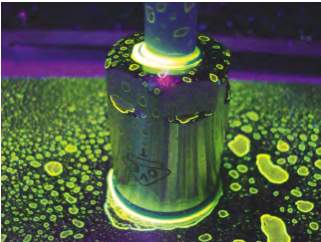
Figure 11. Rittal stainless steel, hygienically-designed cable gland: after wiping – weak.
