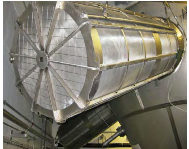
Figure 3. Spray dryer protected by the flameless venting device Q-Rohr-3.
