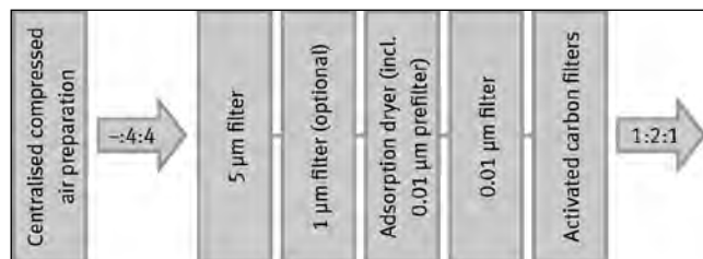
Figure 4. Classification of compressed air quality to ISO 8573-1:2010: [1:2:1].
