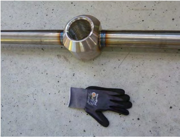
Figure 9. Friction welded stir shaft (1.4404).
