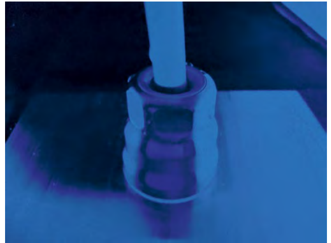
Figure 21. Hummel cable gland: after pressure rinsing – excellent.
