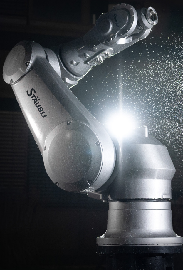
The TS2 HE SCAQRA robots are ideally suited for pick-and-place Q, handling and sorting tasks, thus completing the product range for humid environments.
