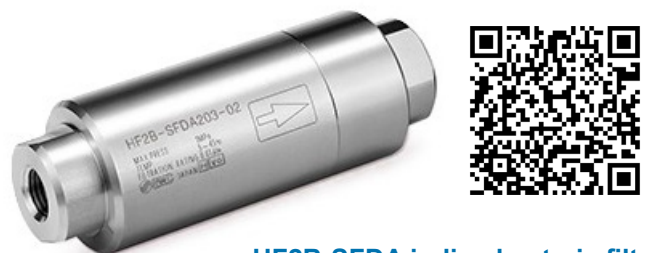
HF2B-SFDA in-line bacteria filter for safe food air: 99.99% filtration (0.01 µm), LRV ≥ 9, FDA-compliant, NSF-H1 lubrication, 500 l/min flow.
