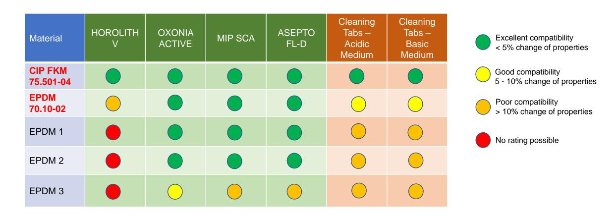
**PERTEC®** CIP FKM shows extremely high performance with very aggressive solvents and acids and achieves by far the best test results in keeping the mechanical properties.
