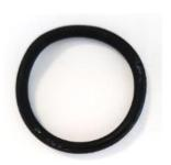
EPDM 70.10-02, slight deformation but no cracks
