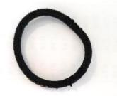
EPDM 1, strong deformation and cracks
