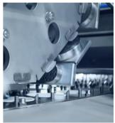
Softwaremodul Anti-Slosh: Fast reduction of swinging liquid/fluid to a minimum by a special control of motion
