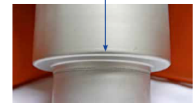
Figure 1. Pressed body. The arrow points to the smooth bottom surface of a pressed drain body where absence of welds has eliminated a typical hygiene troublespot.
